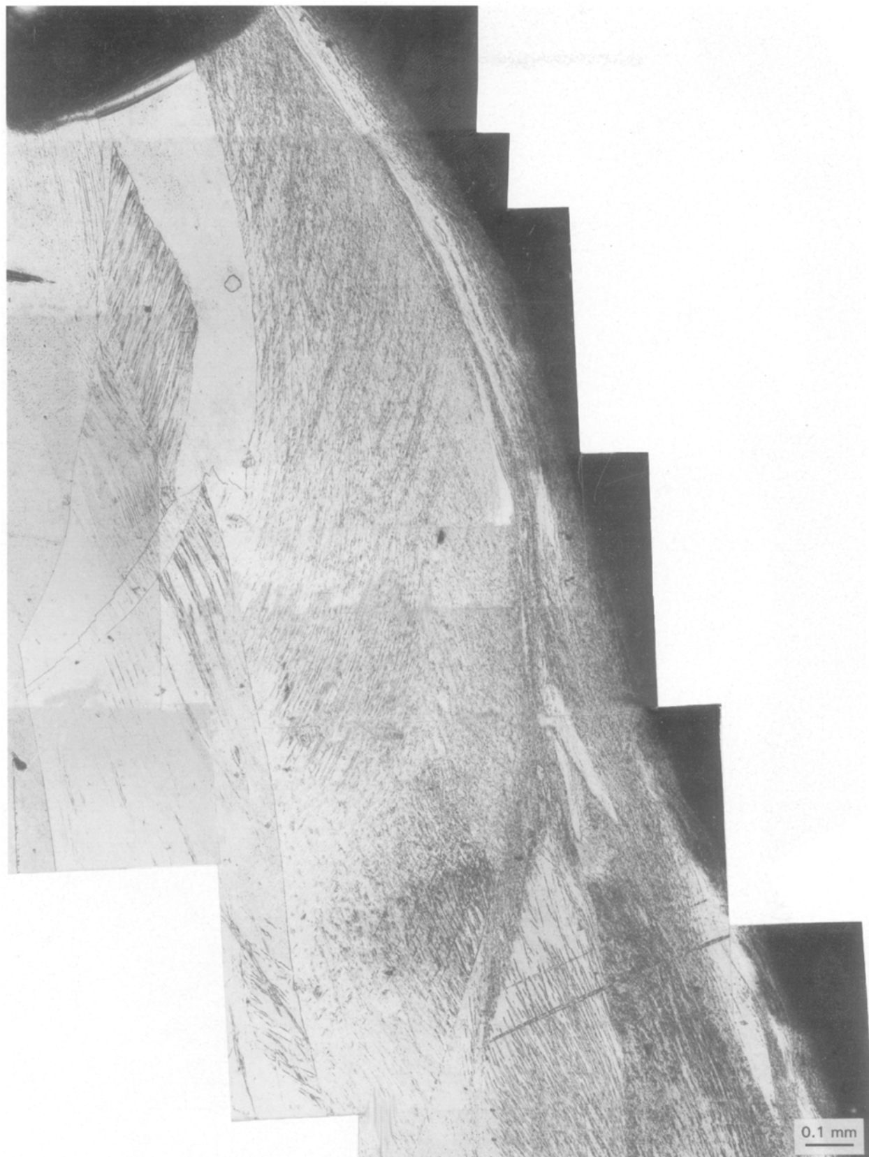
Figure 4 Enlarged view of the crater wall/rim-related region in the large-grained (annealed) crater marked with the arrow at "r" in Fig. 3a. Note the propensity of microbands in many grains.
