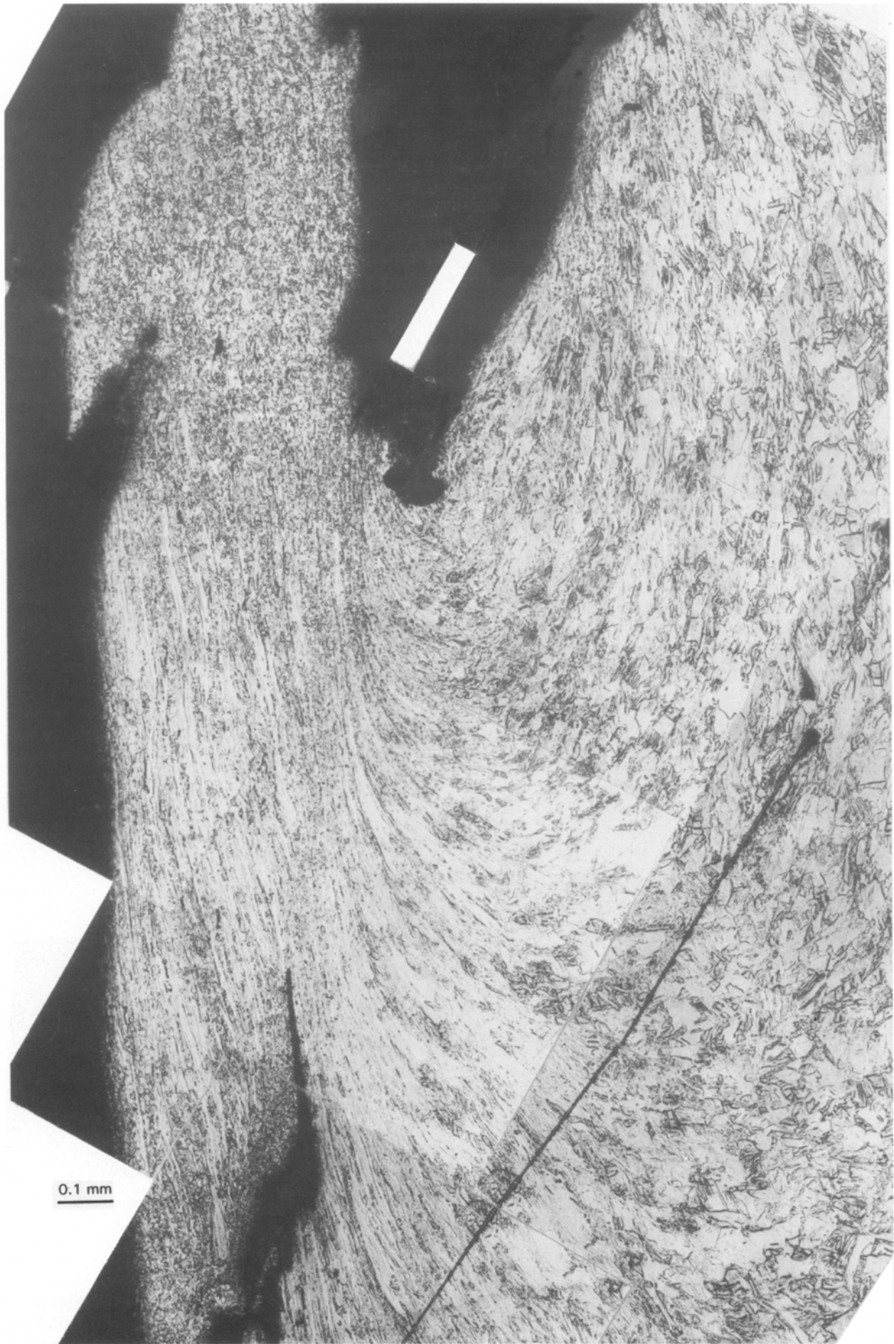
Figure 5 Enlarged view of the crater wall/rim-related region in the small-grained (mill-processed) crater marked with the arrow at "r" to the right in Fig. 3b.
